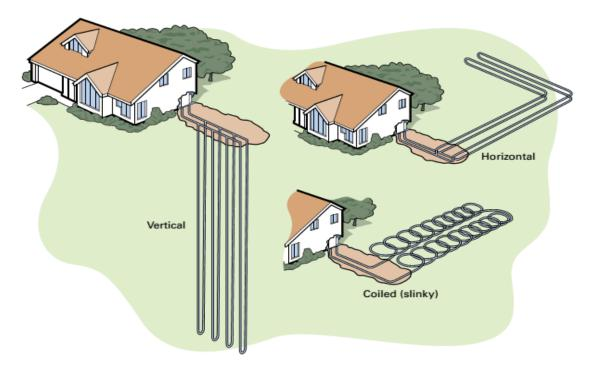
Figure 25: Atypical GSHP ground pipe layouts
