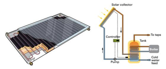
Figure 23: A Typical Solar Thermal Technology
