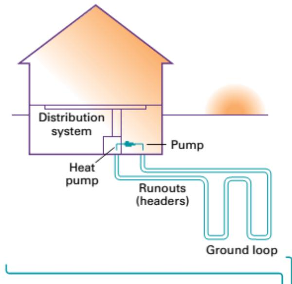
Figure 24: A Typical GSHP Scheme
