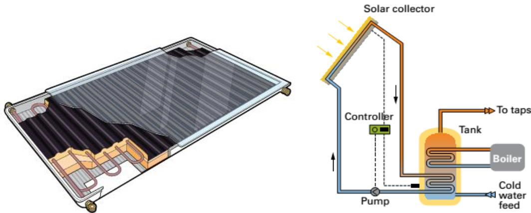
Figure 23: A Typical Solar Thermal Technology
