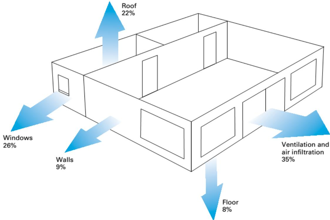
Fig 20: Heat loss from a typical building
