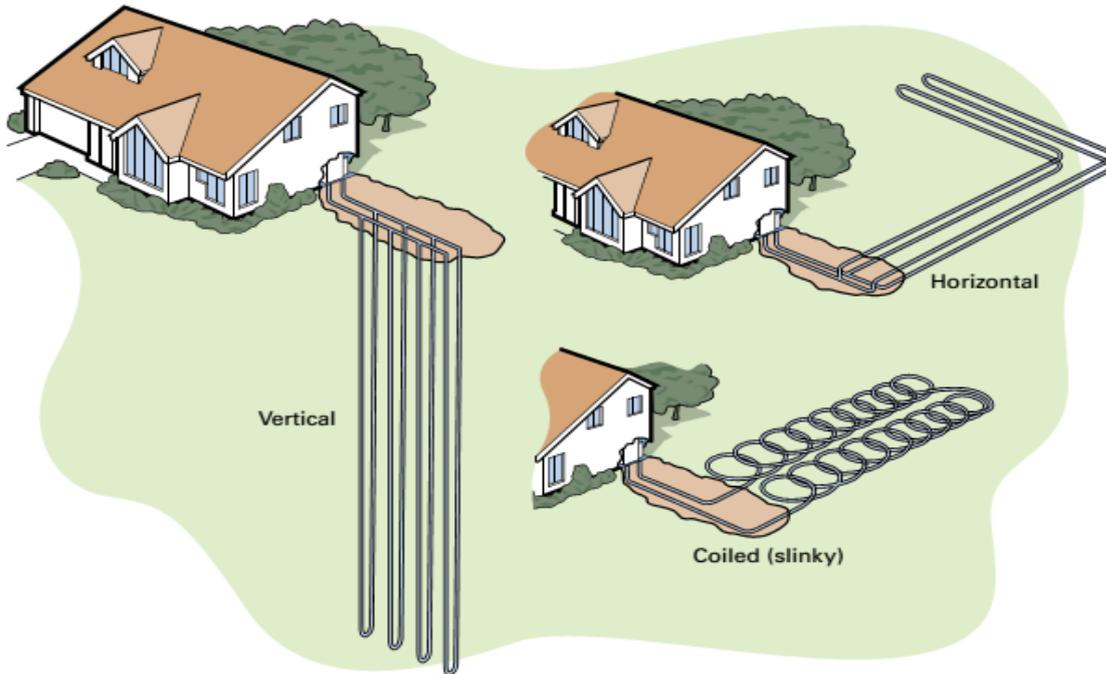
Figure 25: Atypical GSHP ground pipe layouts
